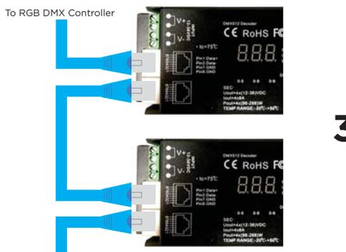
If wiring additional RGB DMX Decoders, connect a CAT-5 cable to the OUTPUT Ethernet port of the RGB DMX Decoder you just installed. Connect the same CAT-5 cable to the INPUT Ethernet port of your next RGB DMX Decoder. Repeat this process for any additional RGB DMX Decoders you install.
