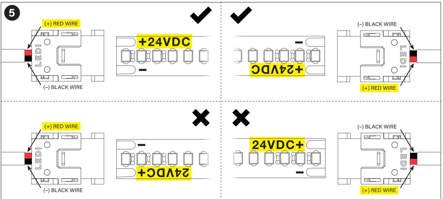
5 For correct polarity, align the connector with the tape light as shown. Otherwise, the LED tape light will not light when powered.
