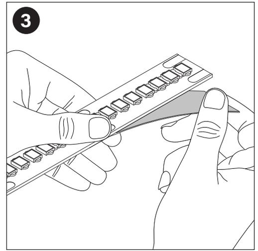
3 Peel back a small portion of the red 3M VHB backing to expose the adhesive.
