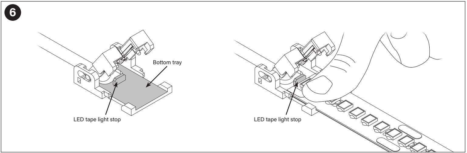
The LED tape light must be aligned with the tray and rest flush against the edge of the LED tape light stop, as pictured above. Once aligned and flush, press the LED tape light onto the bottom tray of the Zeus HD connector.
