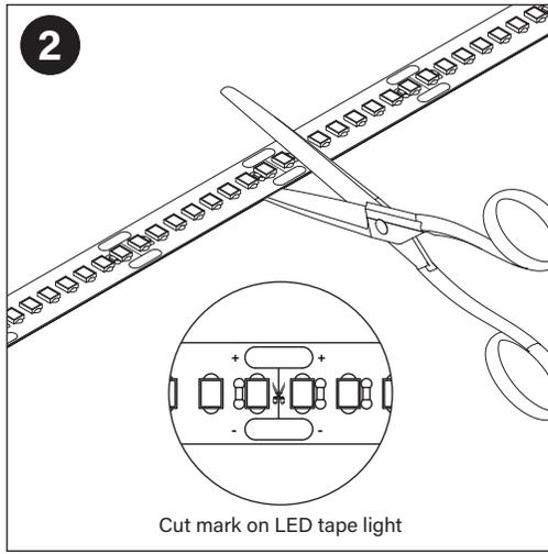
2 Cut the LED tape light to the desired length, at the designated cut marks only.
