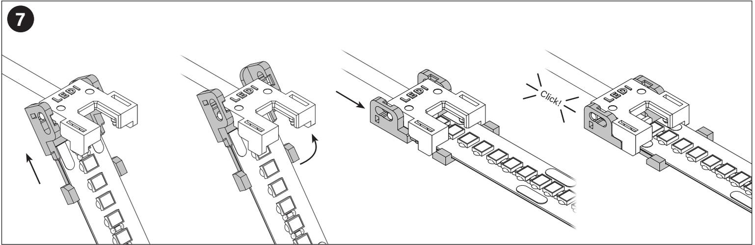
To lock the connector, slide the tray backwards, close the connector, then pull the tray forwards. You should hear and feel a slight "click" when the connector is fully locked.
