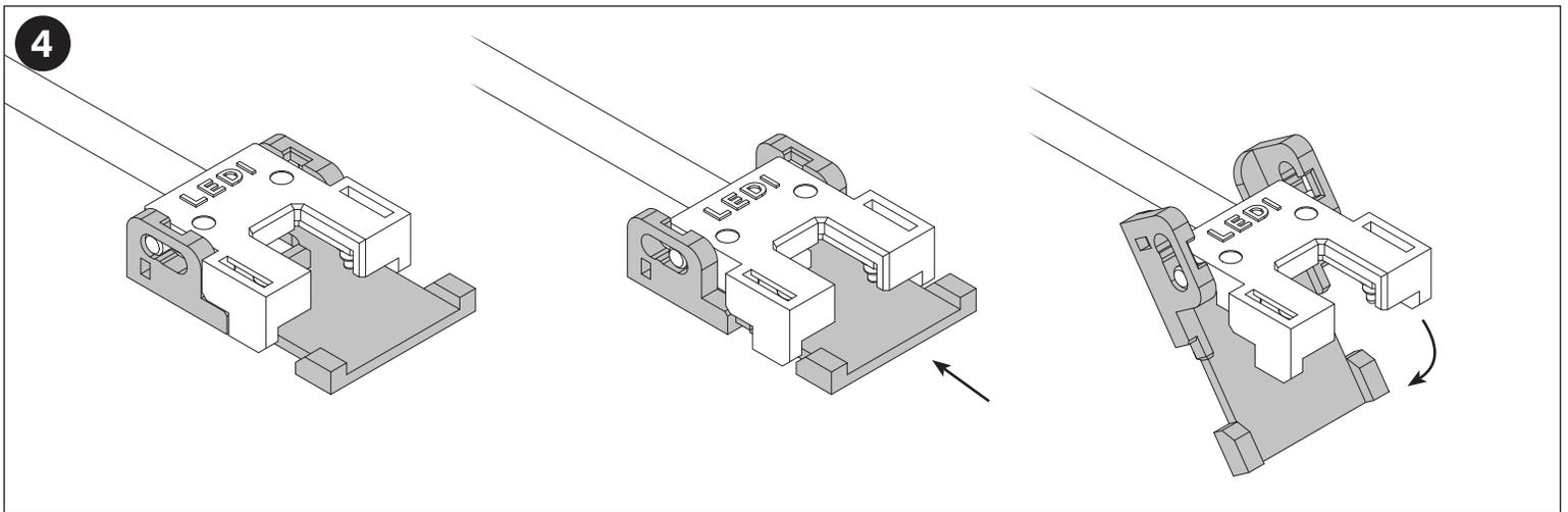
4 Unlock the Zeus HD Connector by sliding the bottom tray backwards.
