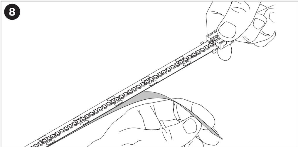
Peel off the remaining red 3M VHB backing to expose the adhesive.
